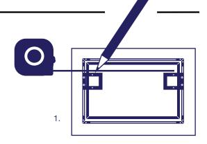
3. Measure the centre of the back of your work (bottom to top) and the distance between this measurement and that of the top of your canvas hangers. This will inform the height at which you will be placing your screws, nails or hooks. If you are working at a height of 156cm and your canvas hangers are 10cm higher than the centre of your work, this will be a drilling height of 166cm.
